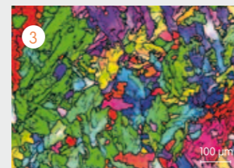
Grain orientation in the BL (coarse microstructure with preferred grain orientation) before post-welding heat treatment.
