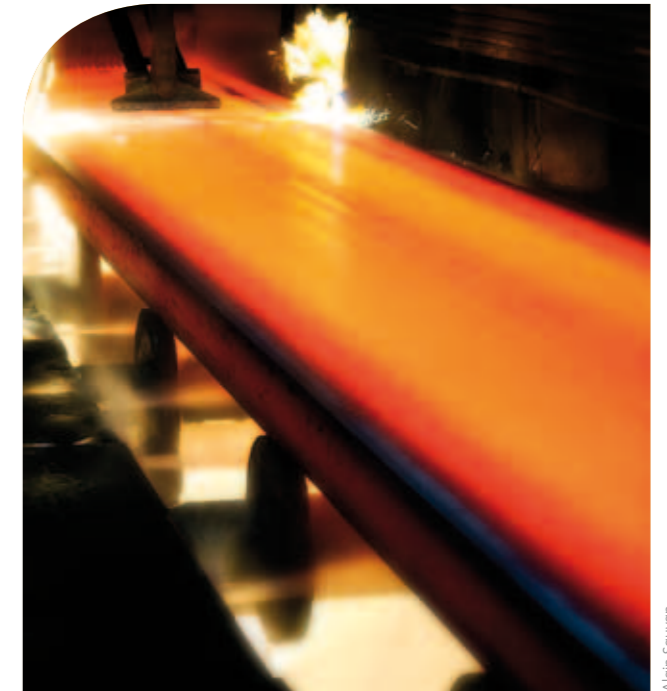
Slab oxycutting at Fos-sur-Mer
