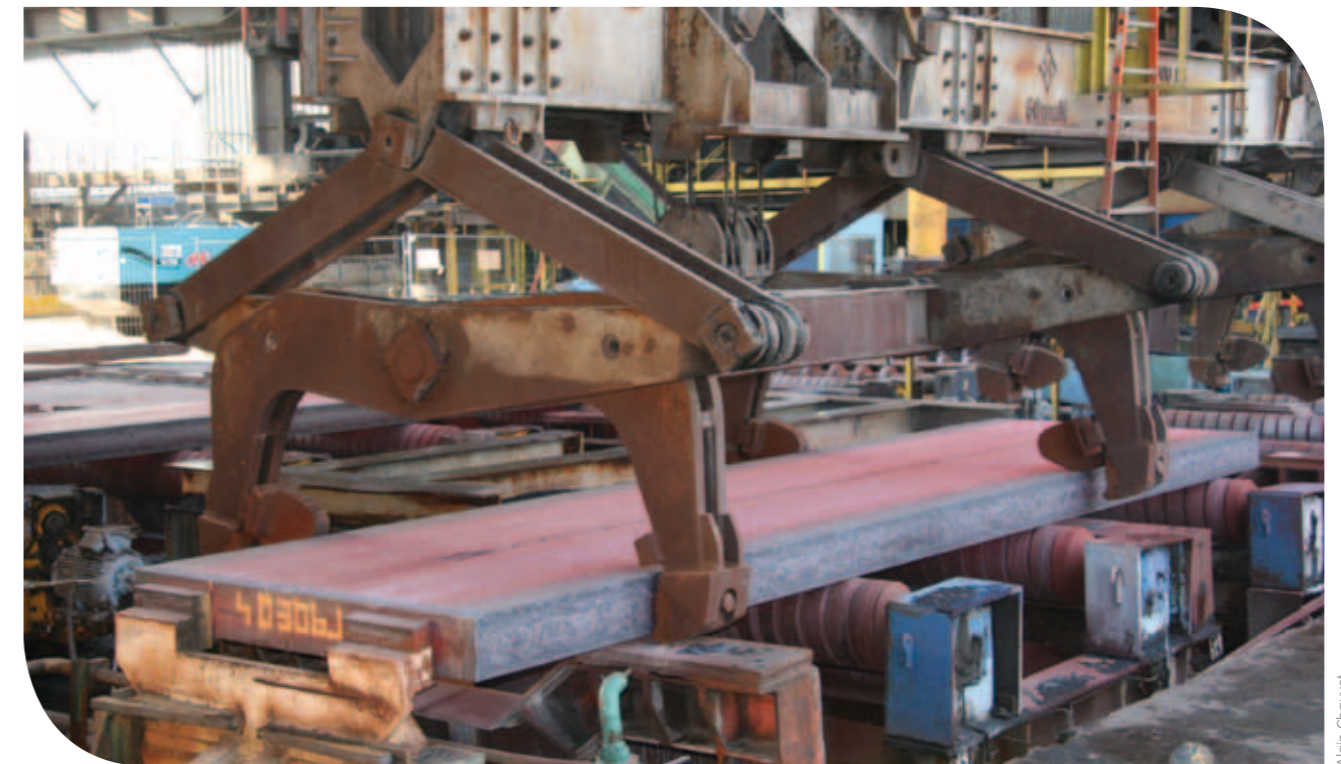
Slab being loaded from the continuous casting exit table after final water spray cooling (Fos-sur-Mer)
