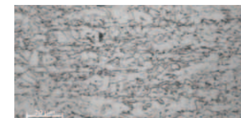
2 - X80M-PSL2 Thickness = 23.7 mm Optical micrography
