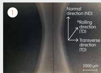
Overview of the weld after Nital etching, prior to heat treatment.
