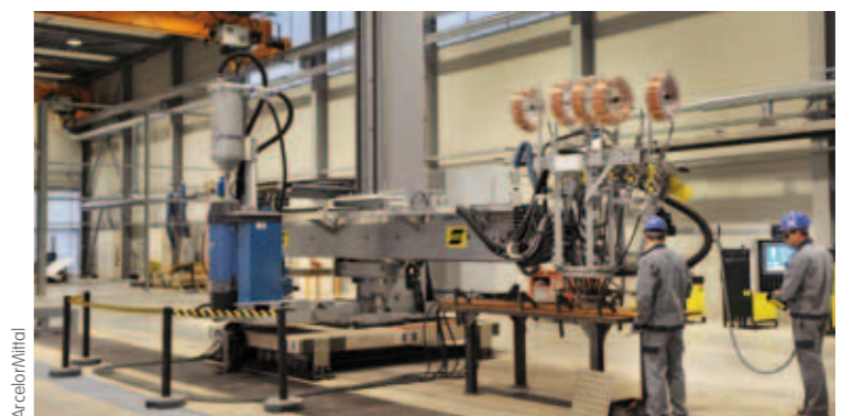
Recently (2011) installed SAW equipment in Zwijnaarde (Ghent)
