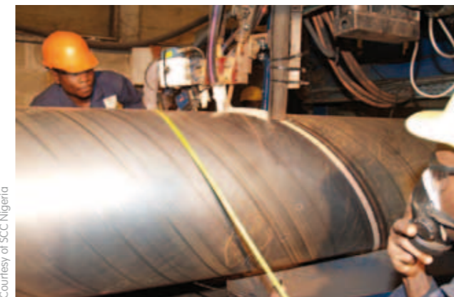
SAWH (left) and ERW (right) welding heads overview
