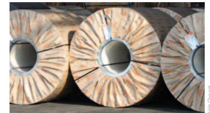
Pickled and oiled coils ready for overseas shipment (Fos-sur-Mer)
